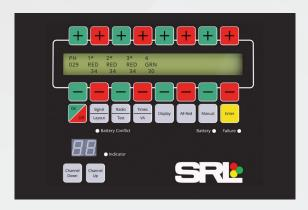
The system will always start on 30s max green and increase by 3 seconds every time the approach reaches its max. If the traffic then reduces, the system will then drop 1 second every time the approach does not reach its max. If the traffic reduces, The max timer will reduce by 1 second every time the max green is not reached.
