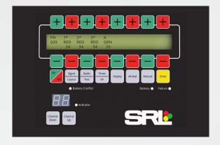
The system will always start on 30s max green and increase by 4 seconds every time the approach reaches its max (which is set to 60). If the traffic then reduces, the system will then drop 1 second every time the approach does not reach its max.
